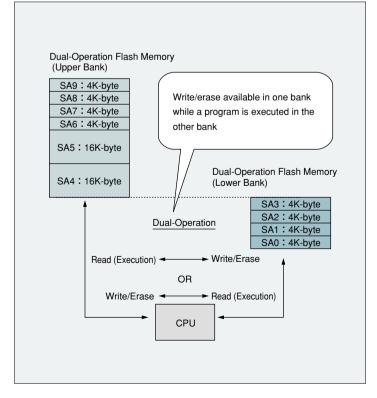
Figure 1 Operation of Dual-Operation Flash Memory-Integrated Microcontroller Series MB90F897
